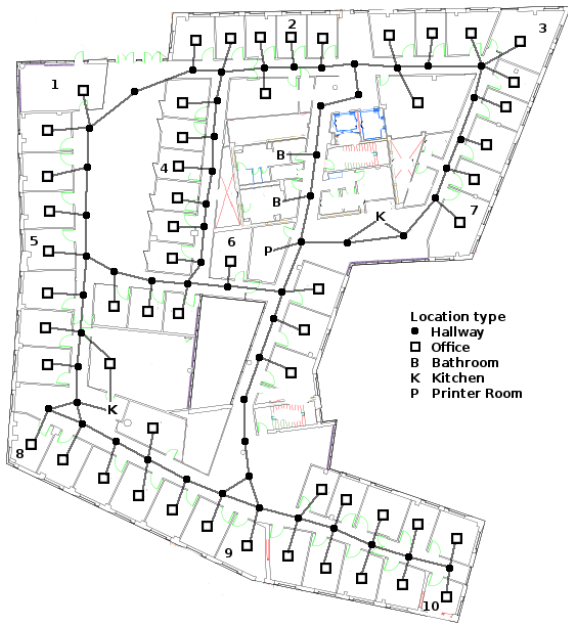
Figure 7: Floor plant considered for the experiments. The embedded graph represents the map given to the planners. The initial location for the experiments are represented by the numbers 1, . . . , 10.
