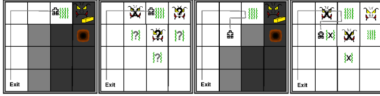
Fig. 4. Four maps representing two situations in the Wumpus World. The first and the third maps show what the agent already knows about the environment: white squares represent visited positions; black squares represent not visited positions; and grey squares represent not visited positions which were inferred to be safe. The second map shows the agent’s hypothetical reasoning about the first map, and the fourth map shows the same about the third map. Squares labelled with “?” denote hypothesis; squares labelled with “X” denote a false hypothesis.
